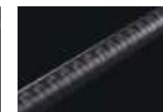
The Cross tape material is used in the blank weave to reinforce and increase sensitivity in the butt section of the rod.
