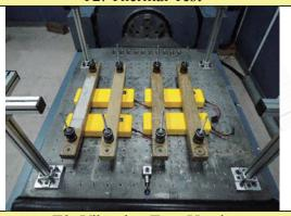
T3: Vibration Test: Y axis
