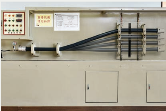
管體剪斷試驗 Cutting Test for PVC-U Pipe
