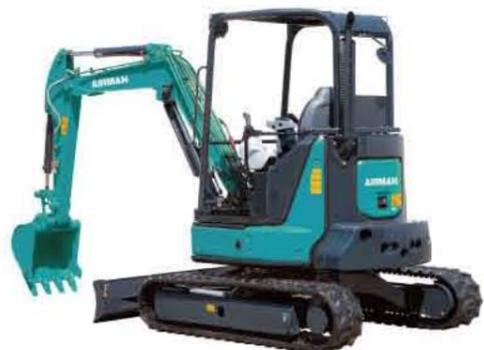
**AX38U-6A** Operating weight **3,710kg** Capacity **0.11m<sup>3</sup>**
