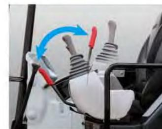
The use of hydraulic pilot type operating levers allows all levers to be securely locked. A neutral engine start mechanism permits engine start only when the lock lever is locked.
