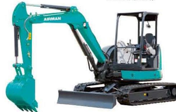
**AX55U-6A** Operating weight **5,210kg** Capacity **0.14m<sup>3</sup>**
