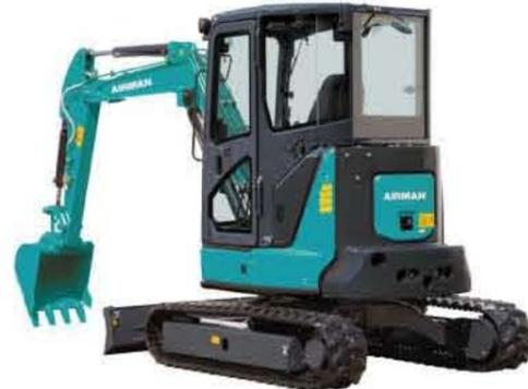
**AX48U-6A** Operating weight **4,540kg** Capacity **0.14m<sup>3</sup>**
