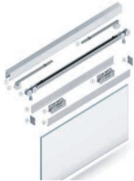
The fitting can be attached directly to the ceiling or by means of a bracket to the wall or ceiling.
