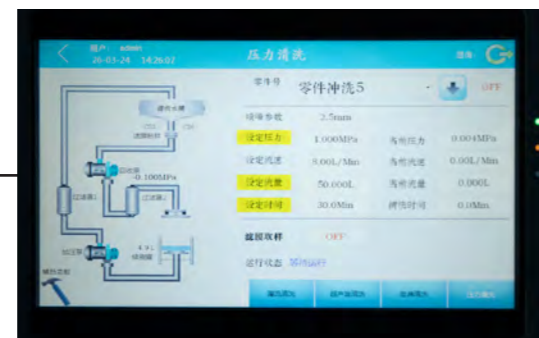
Cleaning / Cleanliness Test ISO 16232 - Cleanliness of Components of Fluid Circuits
