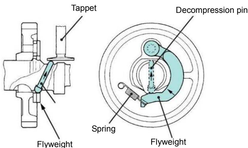
When the cranking speed reaches specified r.p.m., flyweight move to outer against spring force because the centrifugal force applied to the flyweight and the decompression pin coming down.
