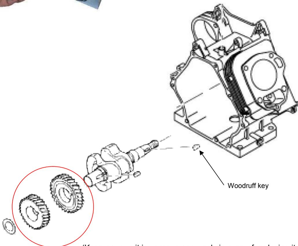
(Keep gear as it is, remove gear, only in case of replacing it.)
