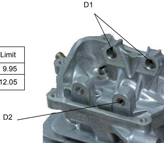
• Rocker arm pin outer diameter (mm)
