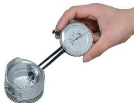
• Piston pin outer diameter (mm)
