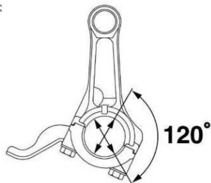
• Clearance between large end and crank pin (mm)
