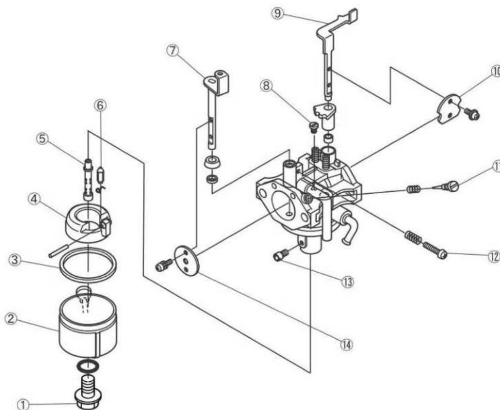
The procedures for overhauling the carburetor are described below.
