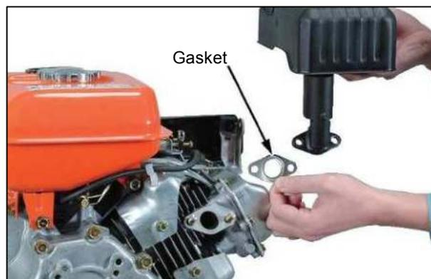
\* Gasket for EK28, 30 it is not necessary to care about its direction.
