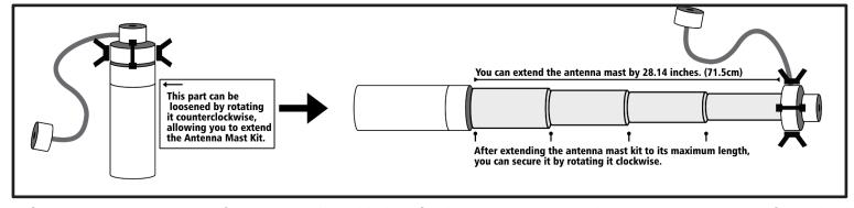
The Large Antenna Mast Kit features an adjustable length, allowing you to extend or retract your antenna for optimal height during installation and convenient storage when not in use.
