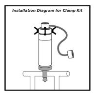
Secure the antenna mount in the ground with the 'Ground-Drilling Kit,' or attach it to a cylindrical object using the 'Clamp Kit.
